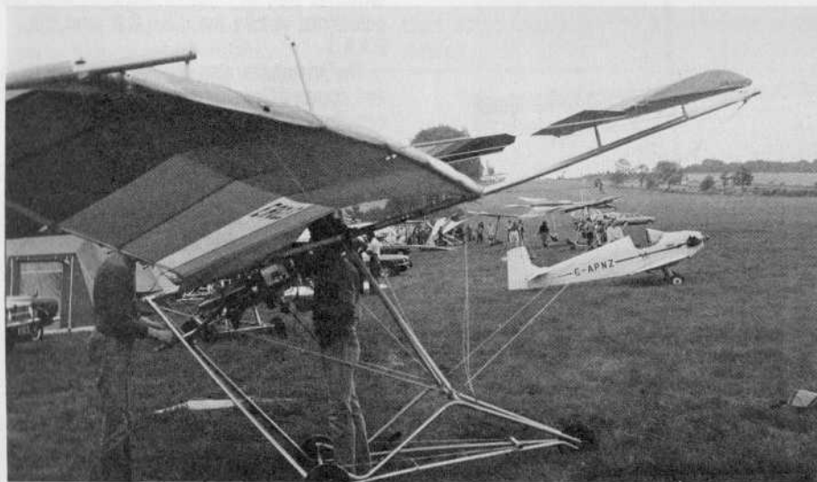
Only three or four years ago, the Turbulent, seen here behind an Eagle being rigged, would have been considered about as minimal as an aircraft could be, having a mere 1600cc's of Volkswagen engine to drag it through the air!
