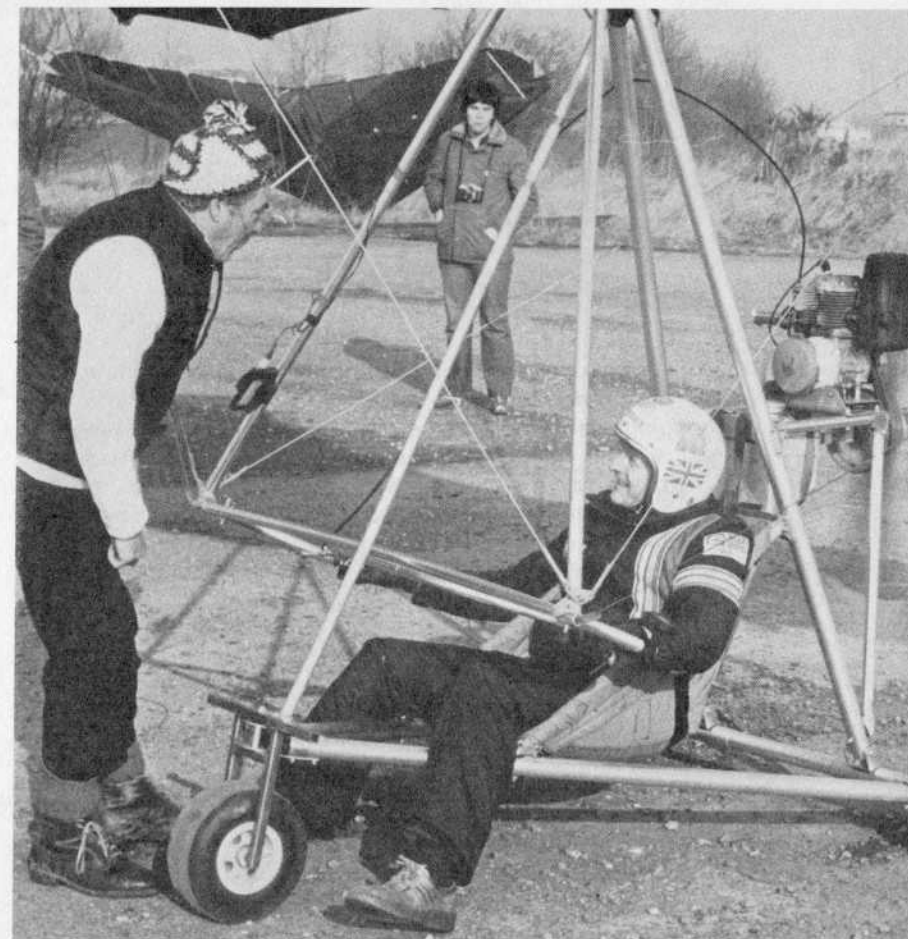
Genial Len Gabriels about to demonstrate his simple Solo-engined 210 cc trike to customer Don Greenbank. Photo by Noel Whittall - 1981
