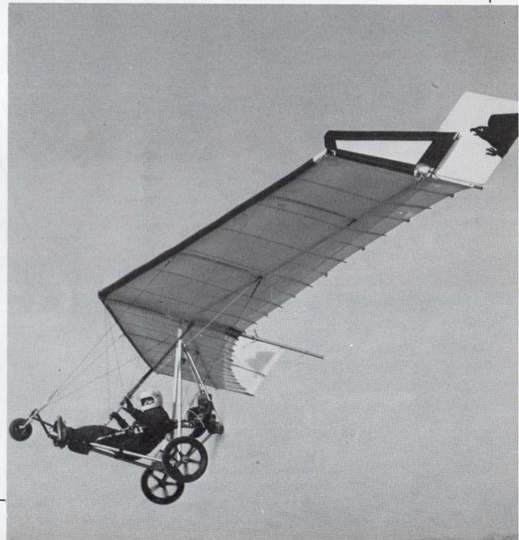
Manta uses a very sophisticated test vehicle, employing computer stored and analyzed information. (Below) Manta's FoxBat combination of Fledge III on their own trike.
