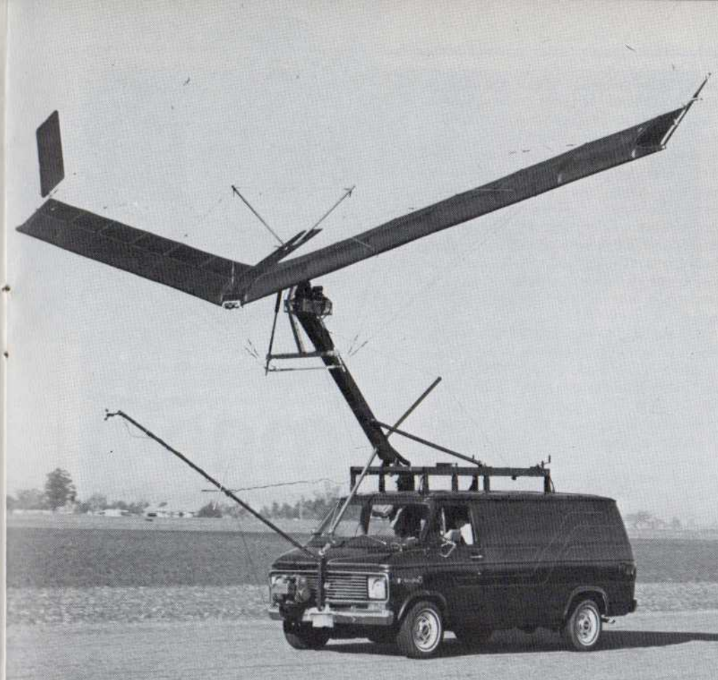
Manta uses a very sophisticated test vehicle, employing computer stored and analyzed information. (Below) Manta's FoxBat combination of Fledge III on their own trike.
