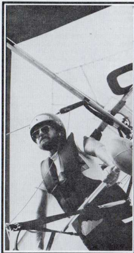
When the tow line passes on one side of the pilot's head, and the release line passes on the other, a dangerous situation can develop.
