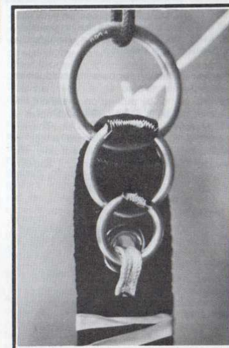
The "three ring" release system, considered by many to be the most fail-safe of systems available.
