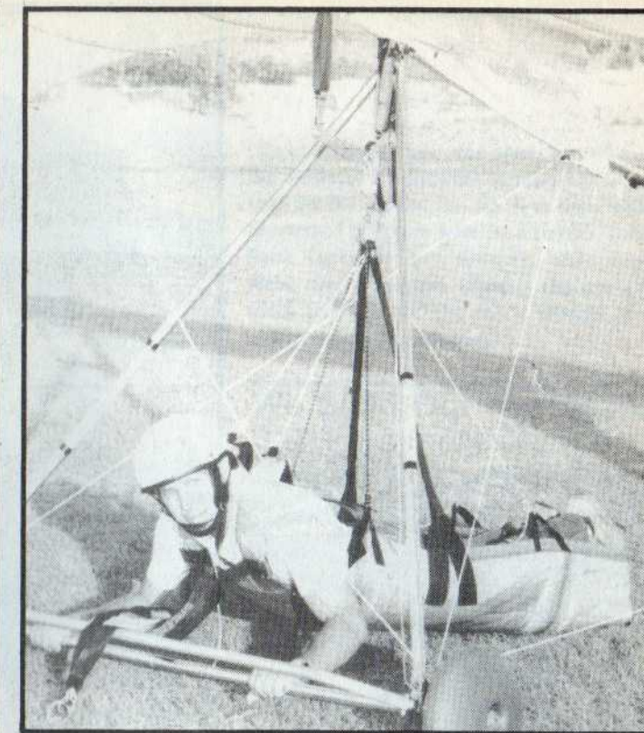
On the left Roland Alexander hang checks the HSNTD, or Roland Connection. Note the forward and locked position of the device. On the right, Roland releases the HSNTD for our photographer. Also note addition of the forward control bar member, which places the control bar in the normal relationship to your body while in 35-40 MPH towed flight.
